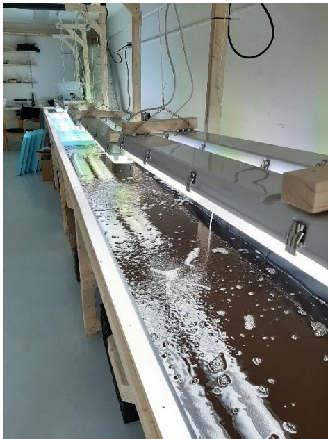
Fig. 12 a – The Deep Water Culture (DWC) at Campus Roslagen when it was filled with water.
