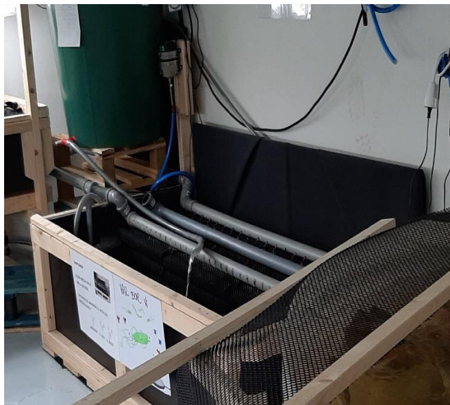
Fig. 11 – The image shows the aerator in the biofilter and a temporary tank used to fill in the sump with tap water (about 10 % of the total volume of water evaporates every month)
