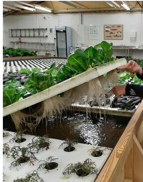
Fig. 12 b – DWC system at Johannas Stadsodlingar (Sweden), showing the plant roots.
