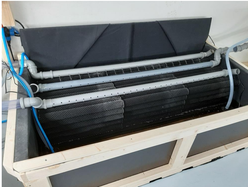
Fig. 10 – Biofilter installed in the sump tank. The biomodules chosen are used for on-site wastewater systems.
