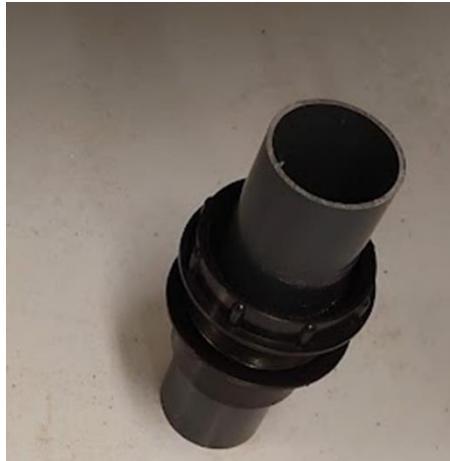
Figure 3. outlet fitting glued to 50mm PVC pipe
