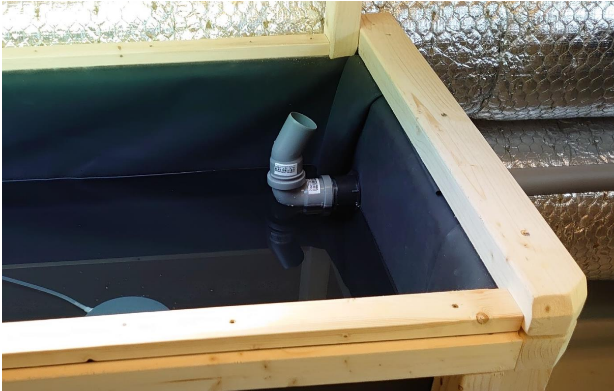
Figure 9. DWC outlet. The height of the water in the DWC is easily adjusted by changing the angle of the grey 50mm pipes. In this picture the DWC is not completely filled. During operation the water level in the DWC is just above the opening of the grey pipe, where the water overflows to the outlet and back to the sump.
