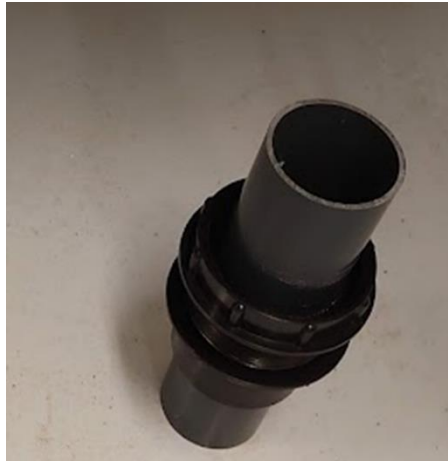
Figure 3. outlet fitting glued to 50mm PVC pipe
