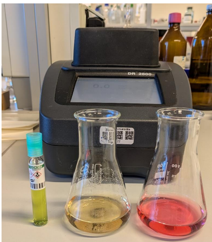
Figure 3. Measurements done for the monitoring of (from the left) ammonium, nitrates and nitrites using Hach DR2800 spectrophotometer.
