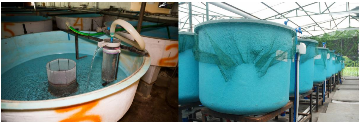
Figure 9. Fiberglass fish tanks are used for fish cultivation in aquaponic systems.
