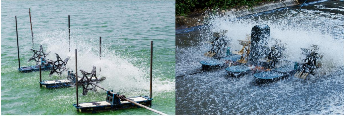
Figure 20. Paddle wheel aeration devices in large-scale aquaculture units.
