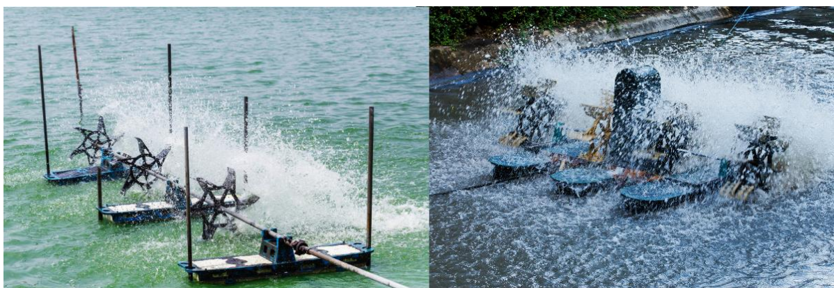
Figure 20. Paddle wheel aeration devices in large-scale aquaculture units.
