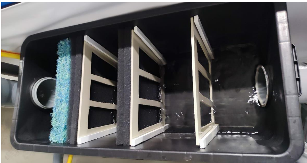
Figure 12. A mechanical filter for sludge removal in an aquaponics system.
