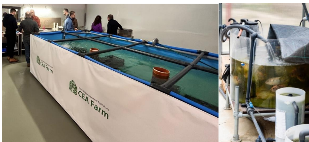
Figure 8. Plastic tanks and containers used for fish cultivation in an aquaponics system.
