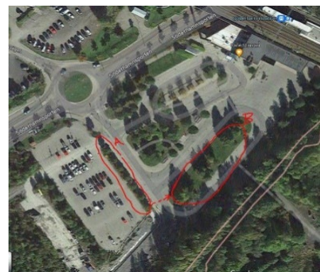
Figure 13 Options A and B in both parking lot/green stripe and on-line water quality monitoring station (A) with construction of the detention area (for water treatment) (B).
