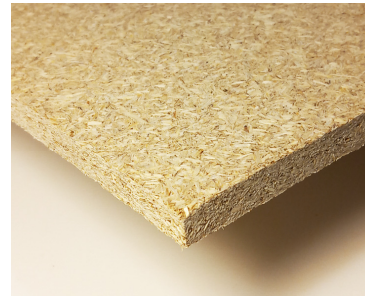
Dense board, 10 mm, 550 kg/m 3
