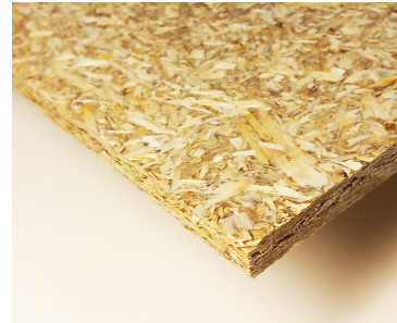
Dense board, 10 mm, 600 kg/m 3
