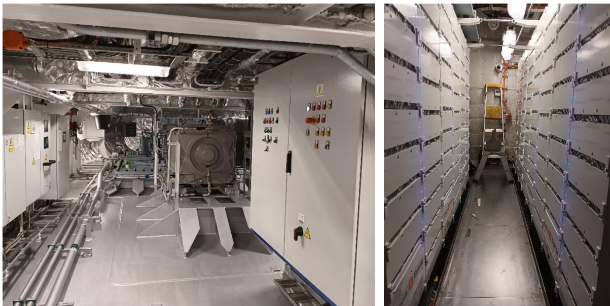
Figure 11. Part of Altera 's engine room (left); Newly installed battery packs on board Stella (right). (Photos: M-L Ojala)
