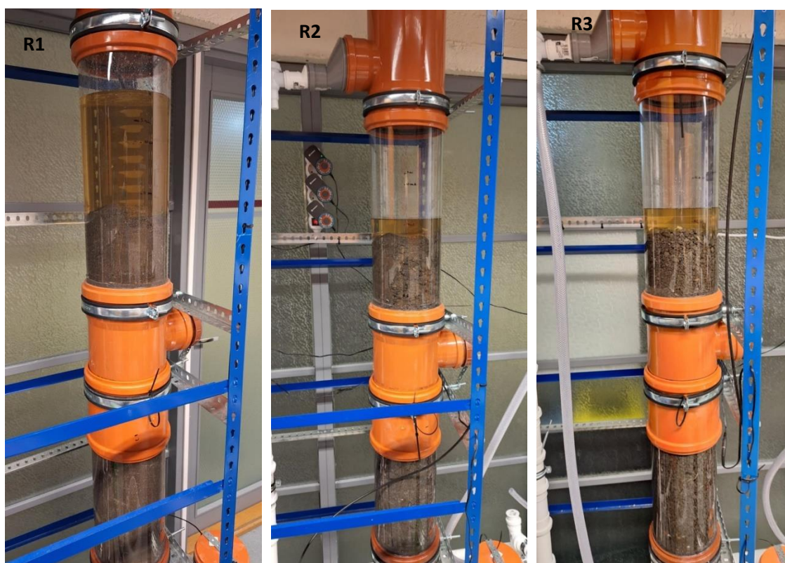
Figure 3. Laboratory scale reactors filled with agglomerates and tap water (leaching test L1): R1, R2 and R3.
