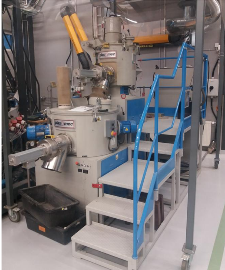
Photo. Agglomeration apparatus. LUT Fiber Composite Laboratory.
