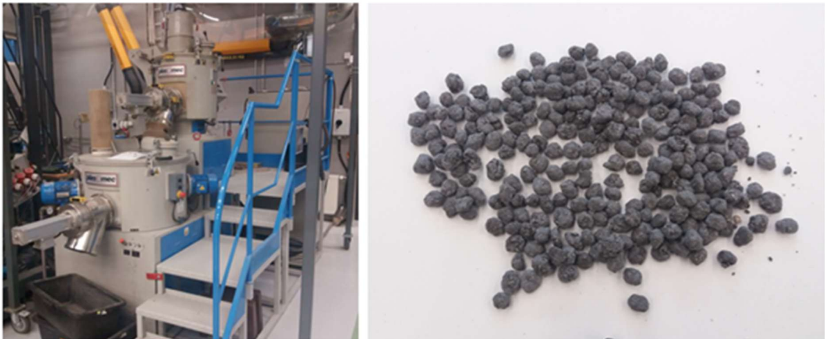
Figure 2.2. LUT University agglomeration equipment ( left ) and produced agglomerated materials ( right ).
