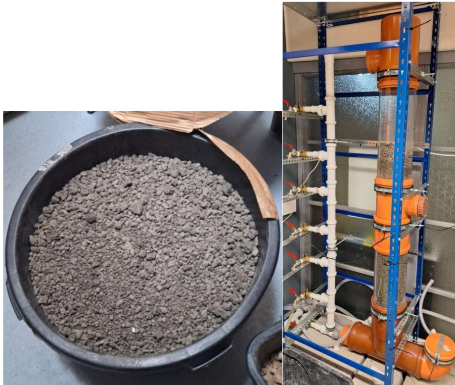
Figure 3.3. Agglomerate sample with a particle size fraction of >4 mm (left) and one of the reactors (right).
