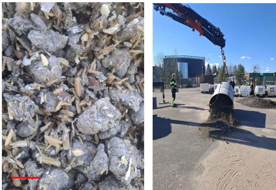
Figure 3.5. Macro image of ACDW ( left ; red bar = 1 cm) and emptying the lysimeters in the end ( right )
