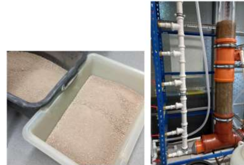
Photo 5. CDW sample with a fraction of 0-5 mm and a fraction of 2.5-5 mm of the packed bed in the third reactor (Reactor 3)
