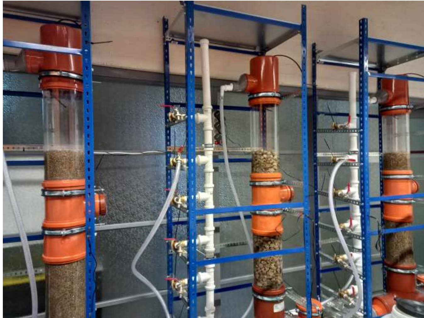
Photo 2. Reactors filled with CDW
