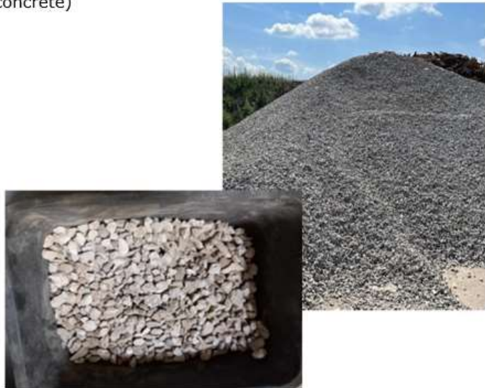
Photo 4. Composition and fraction of CDW used in the second reactor (Reactor 2)
